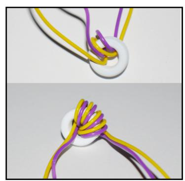
Aim for between 8 and 16 turns of the wire pair around the ferrite core.
