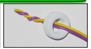
Now you need to wrap the pair of wires around the core.
