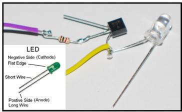
Solder the other leg of the LED (the cathode) to the emitter lead of the transistor.
